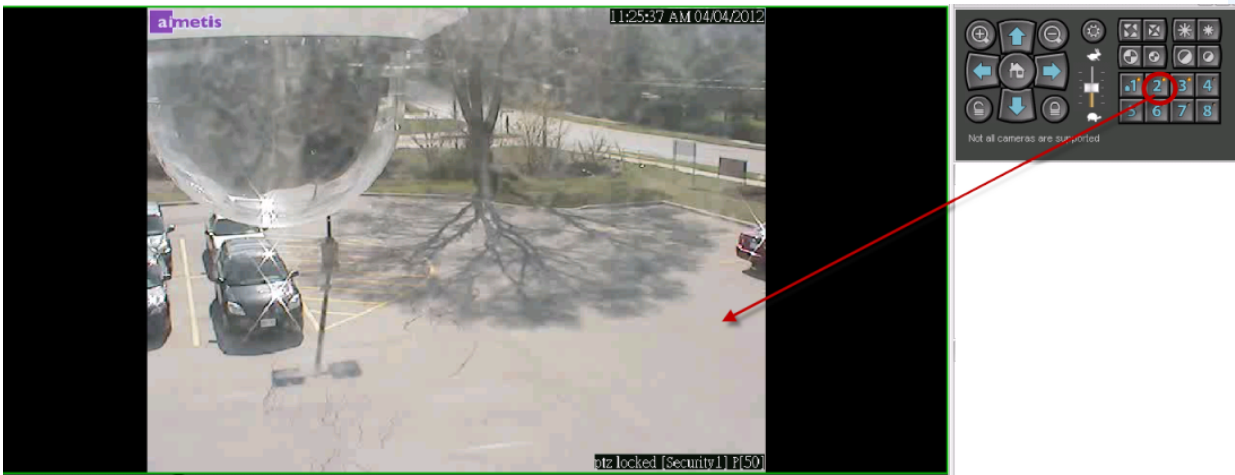
Figure 45. Clicking 2 in PTZ Controls moves the camera to Location 2 in the camera tour
