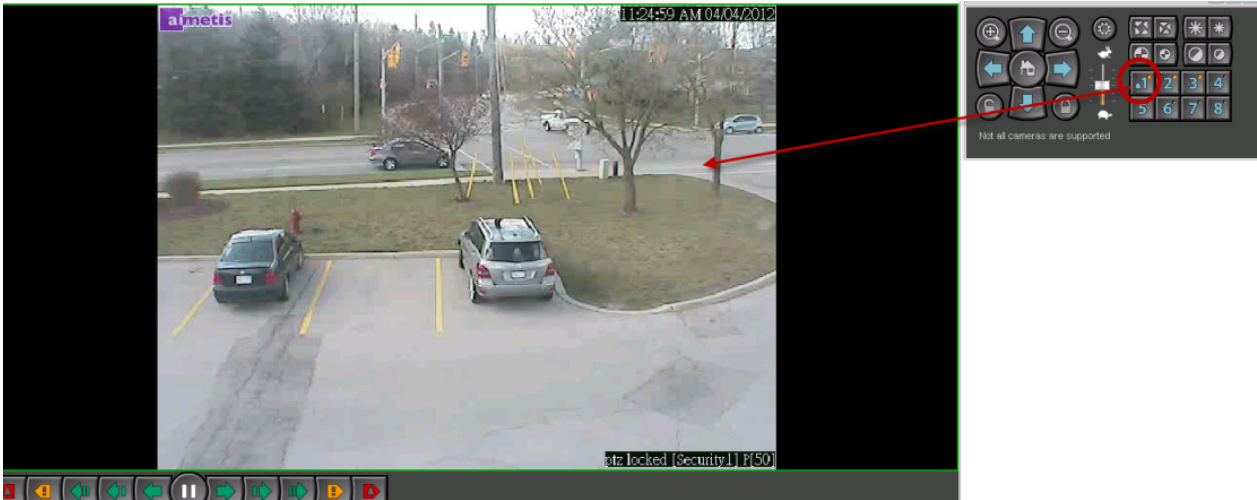
Figure 44. Numbers in PTZ Controls represent camera tour positions
