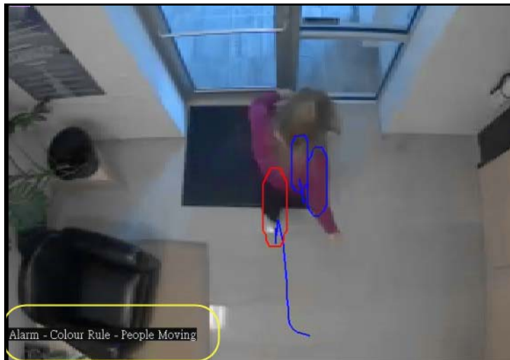
Figure 28. Example of alarm raised on a color rule
