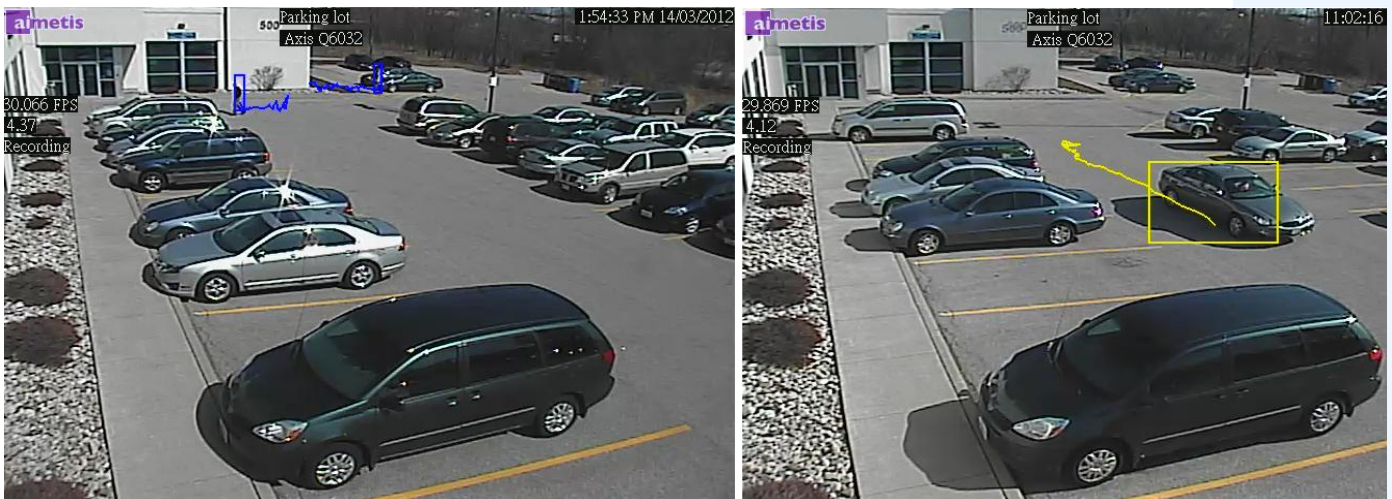
Figure 5. Same parking lot: blue tracking line for person, and yellow tracking line for vehicle
