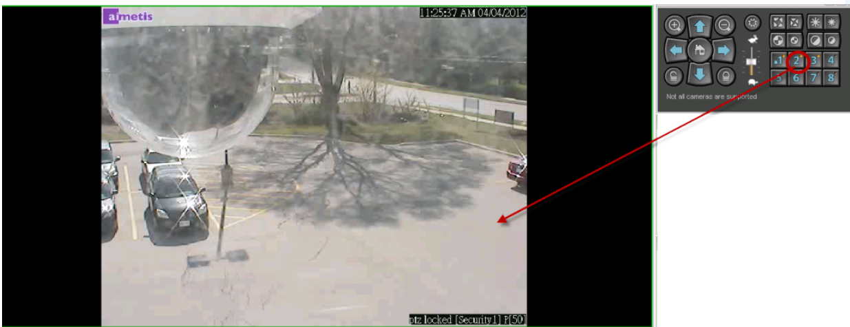
Figure 42. Clicking 2 in PTZ Controls moves the camera to Location 2 in the camera tour
