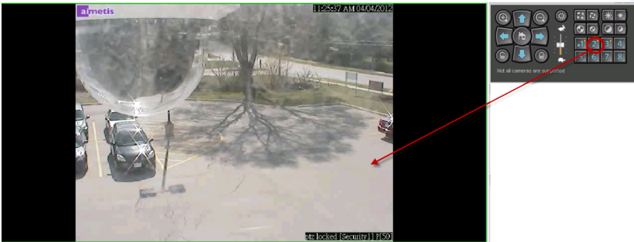
Figure 41. Clicking 2 in PTZ Controls moves the camera to Location 2 in the camera tour
