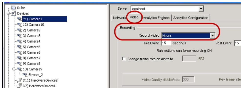
Figure 50. Example of device configuration - Rule Wizard overrides this setting
