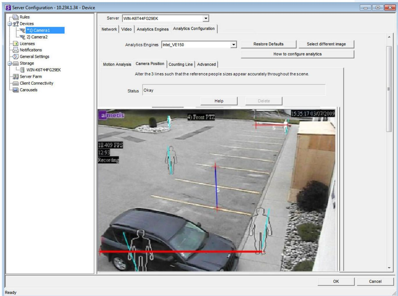
Figure 3. Lines representing perspective in the image
