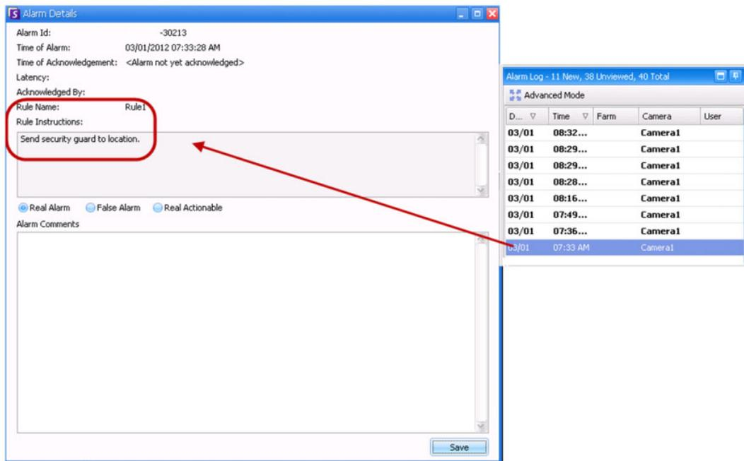
Figure 59. Example – Rule instructions appear in the Alarm Details dialog box
