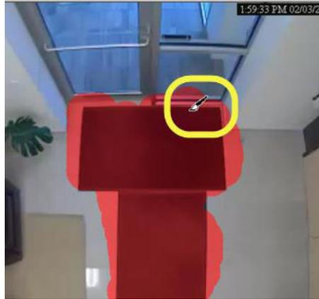
Figure 42. Alarm mask indicated in red
