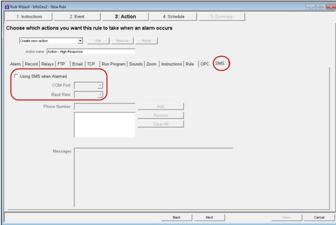
Figure 62. SMS tab in Action screen
