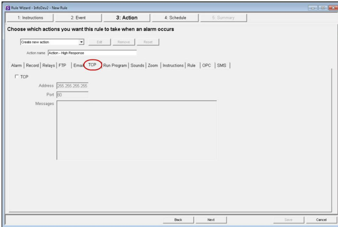
Figure 54. TCP tab in Action screen
