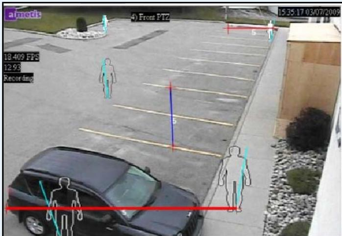
Figure 10. Outdoor Tracking operation mode
